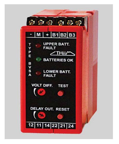
The relay triggers an alarm when an asymmetry is present in the battery packs two halves eg. if a cell in a battery doesn't function anymore. This relay presupposes that the two halves of the battery are identical. For a complete monitoring of the battery, BVSA can be used together with a BMCD (Hi/Low).
